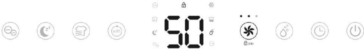
Press the fan speed button for 2s to lock all buttons on the panel with a beeping sound, the same operation can unlock it.
