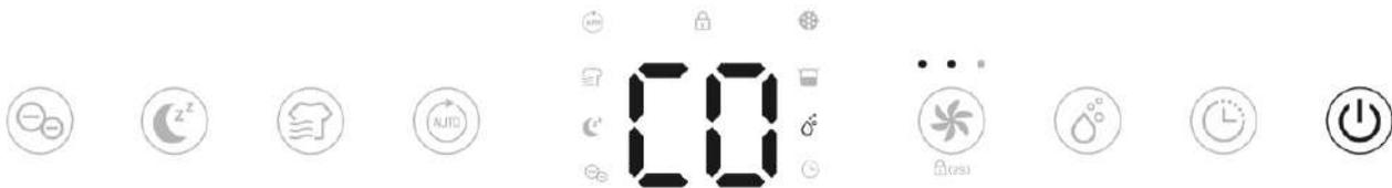
Press the power button once to turn on the unit, the unit runs by default mode on manual continuous dehumidifying with mid fan speed.
