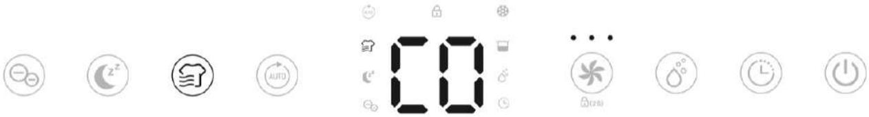
Press the laundry drying button to activate the laundry drying function, the unit runs in continuous dehumidification with high fan speed for 6 hours then switch off automatically.
