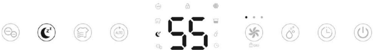
Press the sleep button to activate the sleep function, the unit runs with a designated humidity setting of 55% along with the low fan speed. All indicators will be off 5s after the setting is completed (tri-color light stays on). Touch any button to activate the light, and to operate as usual.
