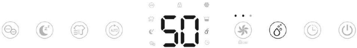
Press the manual button to select your preferred humidity from CO-30%-35%-40%-45%-50%-55%- 60%-65%-70%-75%-80%-CO. CO means continuous dehumidifying regardless of ambient humidity.
